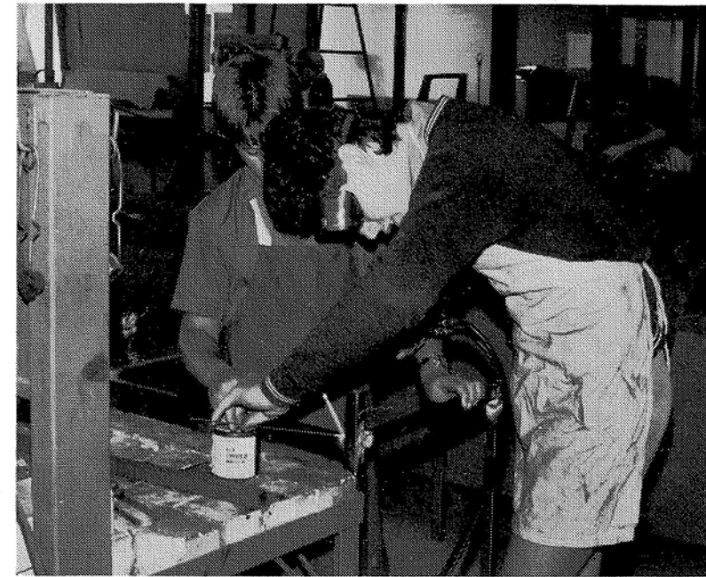
Craig REIMERS and Todd IVEY are using bronze welding to assemble a desk frame.
