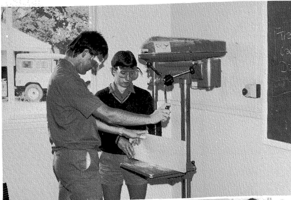
Geoff BARR is assisted by Peter JENNINGS, as a dowel joint is being machined on the drill press.
